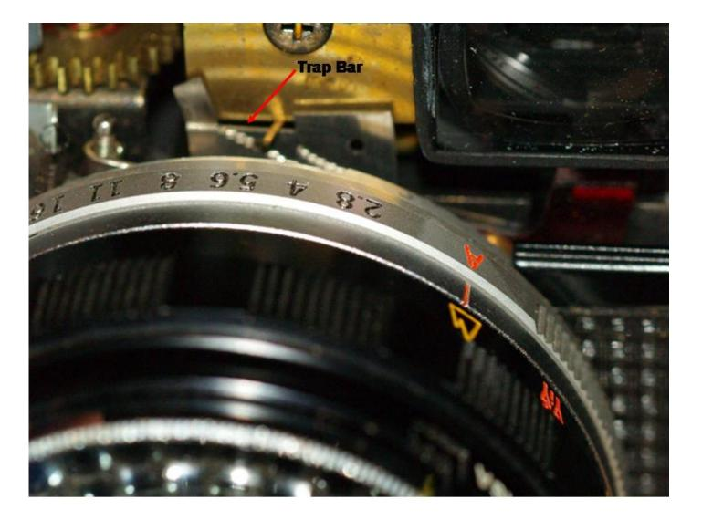
5. Once you have verified that the problem is not with the cell or the meter, it is time to remove, clean and lubricate the aperture blades. You can desolder the hot shoe wire to set the top aside and out of the way. This makes the camera easier to handle, but is not necessary as long as you are careful. Now remove the bottom plate. This is held on with two screws. Put the two little screws in the second cup of the ice cube tray.
