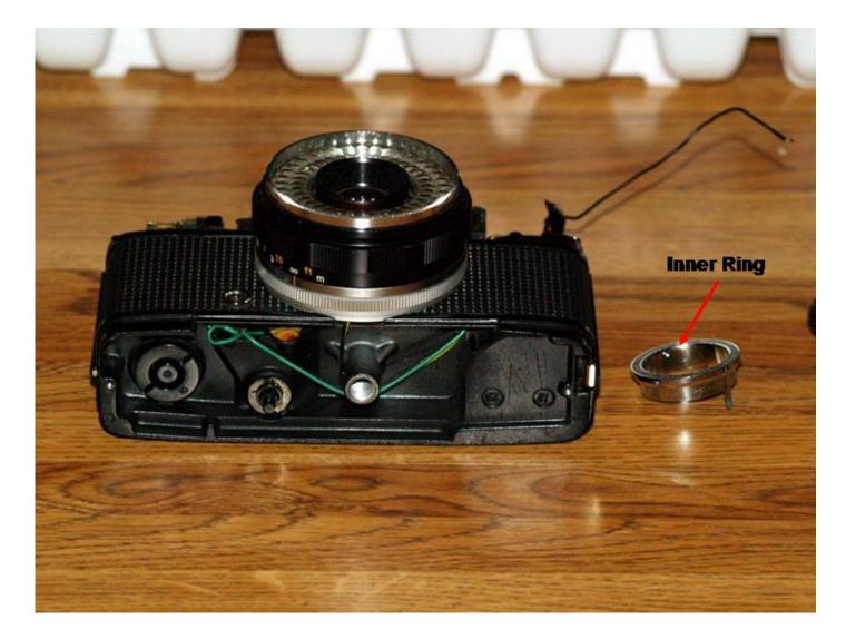
7. Note the position of the front lens element. Use a red marker to mark the 12:00 position. Then just to make double sure, screw the lens in the whole way and note how far it turned. In the picture below the lens turned to about the 2:30 position.
