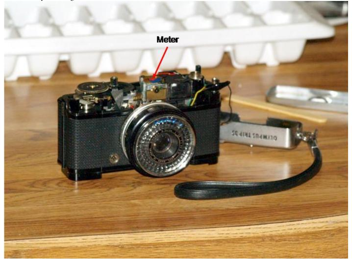
2. The meter needle is just below the brass plate. With no light shining into the cell, the needle will be fully to the left, up against the viewfinder.
